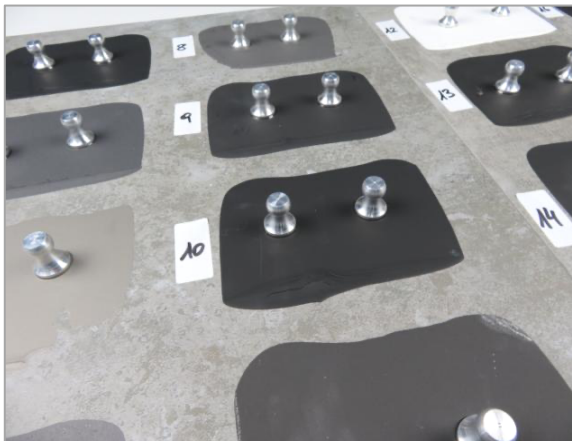
Figure 3: Shielding paint with two stamps each before testing the adhesive tensile strength
