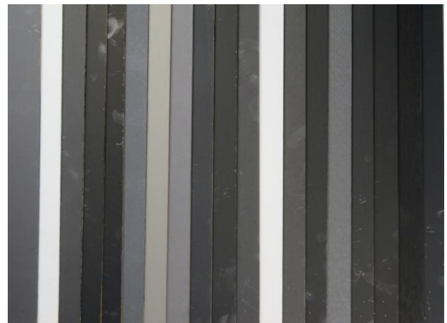
Figure 2: Shielding paint shades after one coat. The two white bars come from a white wall paint with special shielding additives: AegisGuard LP and PEN-YANG Biologische Farb- und Putzbehandlung (fine quartz powder)
