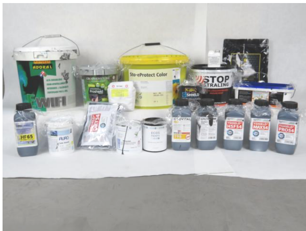
Figure 1: “Group photo” of shielding paints tested and additives for standard paints
